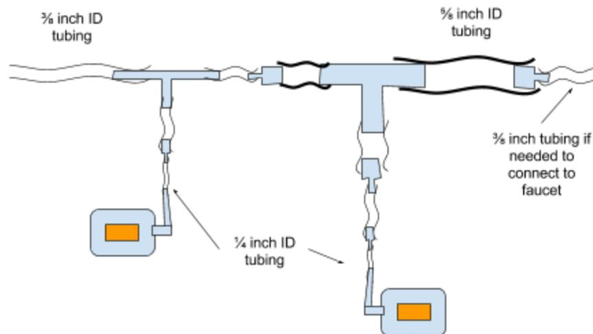
5. Connect one end of the tubing apparatus to the faucet. **Hold** the other end so that water discharges to a sink.
