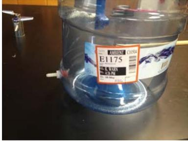
¼ inch tubing connector mounted in side of 5 gallon jug. This step is not easy.
