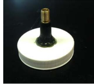
Tire stem valve mounted on jug cap.
